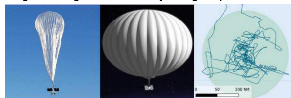
Figure 3: Example heavy category HAB, after launch (left), fully inflated in the stratosphere (middle), and example station-keeping performance over many days (right).
