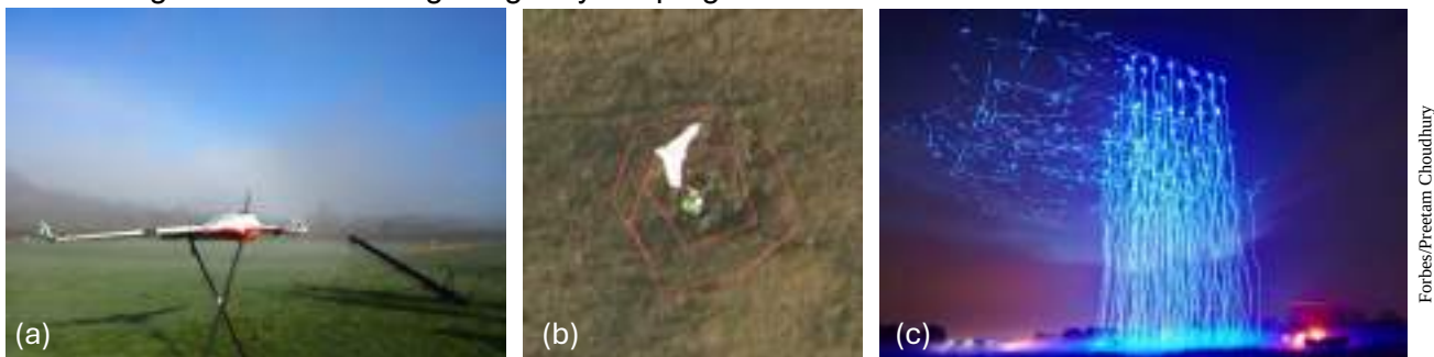
Figure 1. (a) Catapult-launched Skywalker X8, modified for charge release and droplet monitoring in a valley fog. (b) Skywalker X8 viewed in flight from above, over a measurement site. (c) "Shooting star" display event using a swarm of 330g microdrones.
